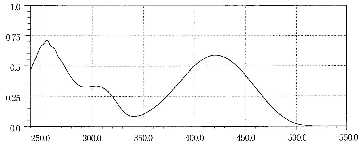
A solution prepared as follows: Dissolve 1.0 mg of Dexamethasone in 10 mL of ethanol (95). To 2 mL of this solution add 10 mL of phenylhydrazine hydrochloride TS, shake, warm in a water bath at 60°C for 20 minutes, and allow to cool.
