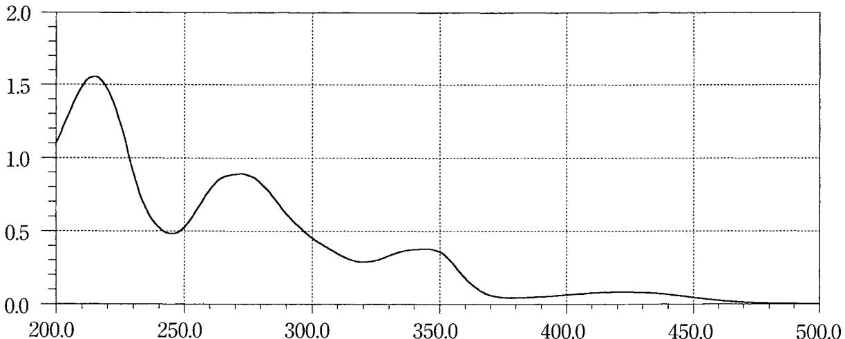
A solution prepared as follows: Dissolve 0.01 g of Berberine Tannate in 10 mL of methanol and 0.4 mL of 1 mol/L hydrochloric acid TS, and add water to make 200 mL. To 8 mL of this solution add water to make 25 mL.
