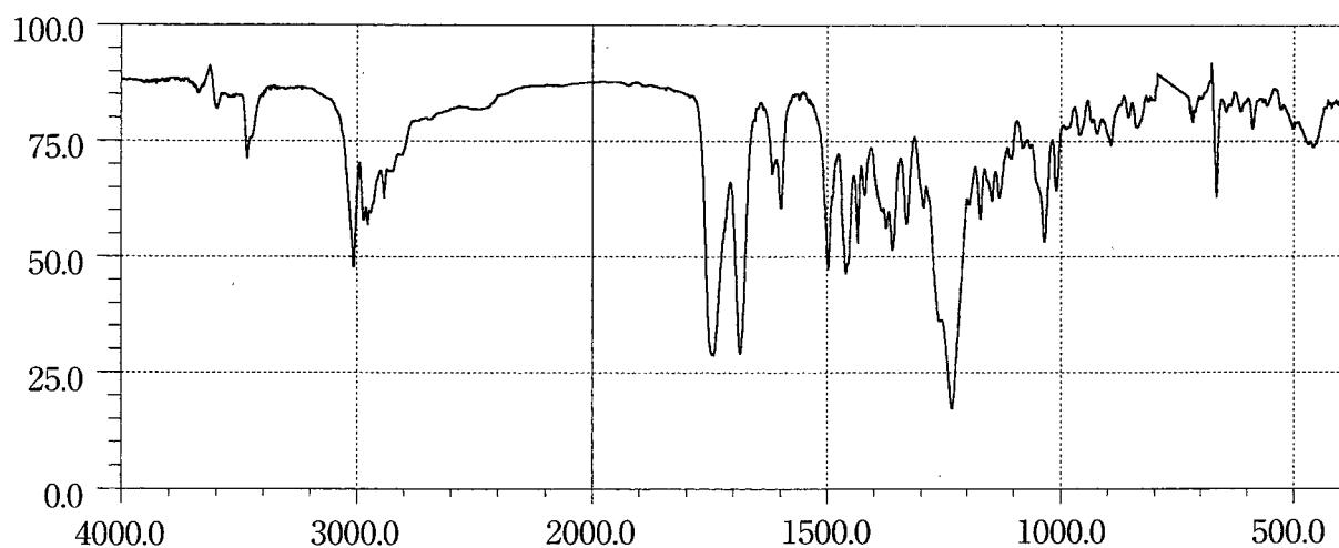
Preparation of sample: Solution method (measured as a solution in chloroform, potassium bromide optical plate, thickness of cell: 0.1 mm)
