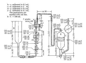
ting B downward, and measure the volume of the residual gas. Repeat the procedure until the volume of residual gas is constant, and designate this as  $V(\mathrm{mL})$ . With fresh ammonium chloride-ammonia TS in C, repeat the procedure at least four times, and measure the volume of residual gas. Calculate V and the volume of Oxygen used as the sample with reference to the gas at  $20^{\circ}\mathrm{C}$  and at  $101.3~\mathrm{kPa}$ .
